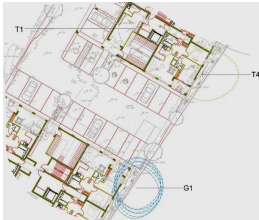
Figure 13: trees requiring removal
