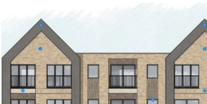
Figure 9: southernmost block – facing brick detailing between the gable features
