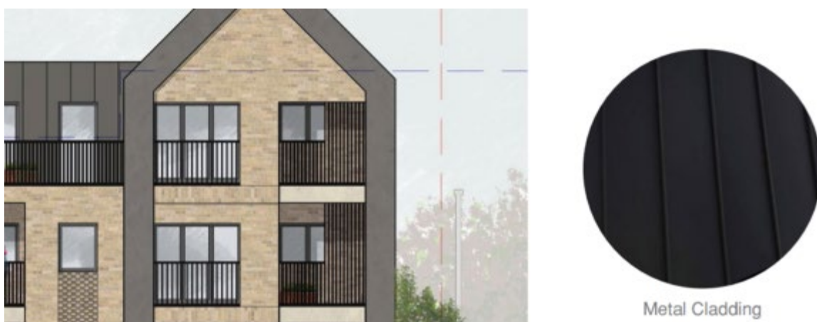
Figure 14: rolled joint metal cladding
